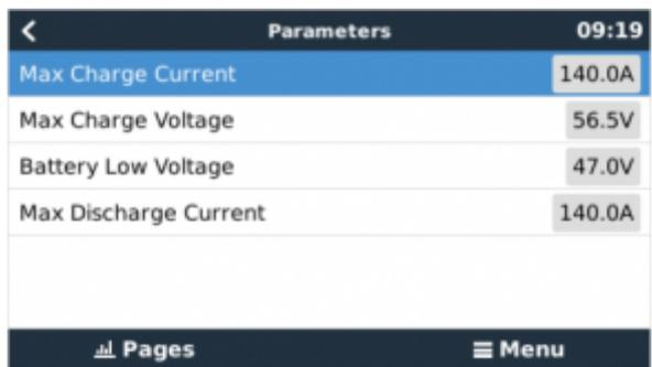
This parameters page is also a good place to check that all batteries are connected and working properly. In normal working conditions, for the 2.5 model, the charge current limit is ~35-50 A per cell. For example, 140A charge current limit (  $140 / 35 = 4$  ) means there are 4 BYD battery cells connected.
